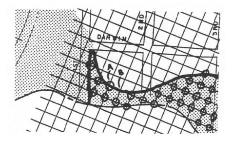
Step 4. Lay the overlay over the area at a different angle and count the number of crosses.
