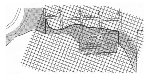
Step 3. Lay the overlay over the area to be measured and count the number of crosses.
